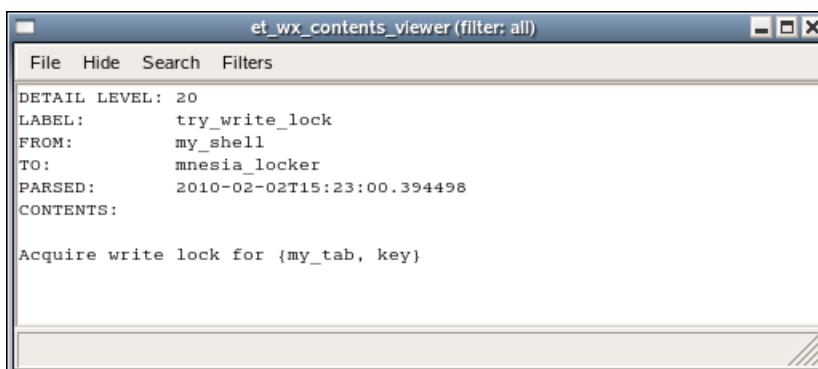
Figure 3.3: Details of a write lock message
