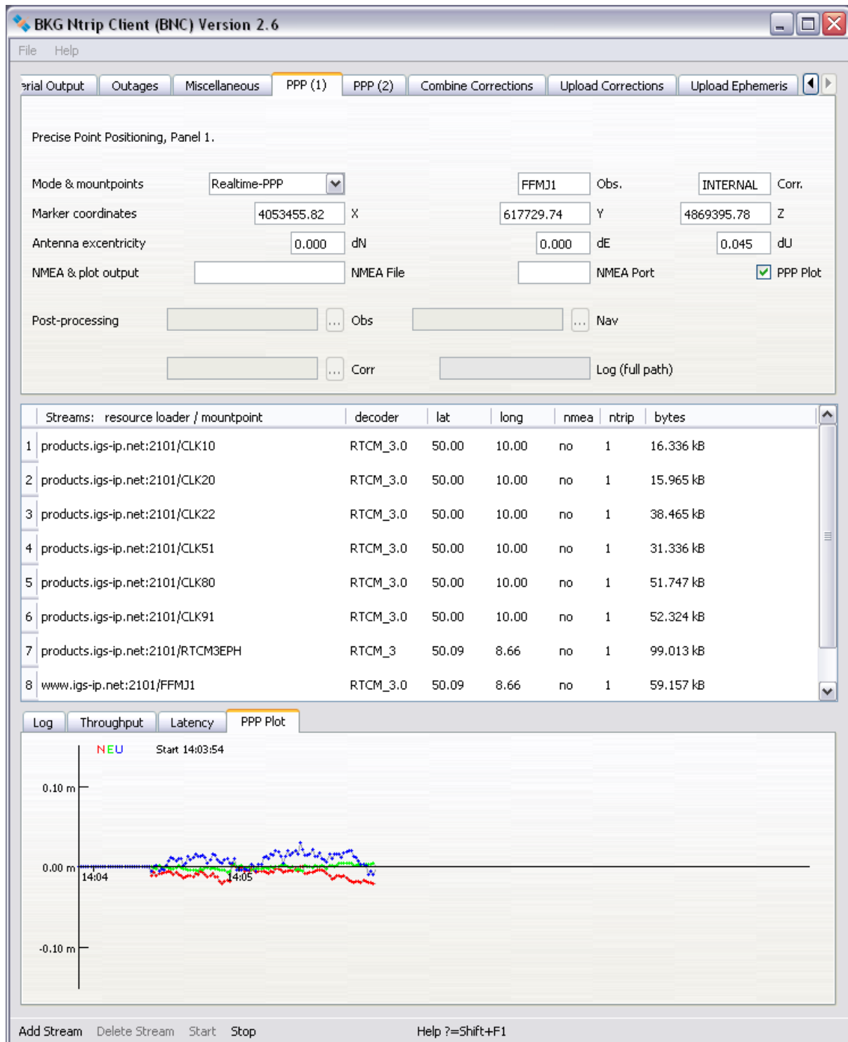
Figure 22: 'INTERNAL' PPP with BNC using combined Broadcast Corrections stream.
